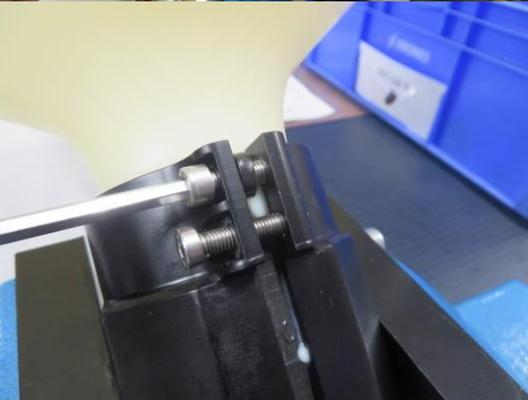
Using a **vise**, clamp the RFC-04-HC / RFC-05-HC to orientate the bottle to the coupling as shown. Clamping the RFC-04-HC / RFC-05-HC will also ensure that the bolts M5x16 can be fitted easily. It is recommended to use **smooth jaws** to prevent damaging the hose clamp.
