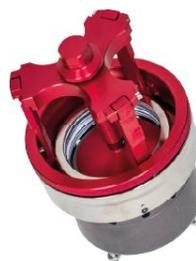
Once the service tool is coupled you can lock the tool by turning the locking ring clockwise. Then you can open the valve fully by turning the shaft clockwise. You can grease or change the o-rings then.
