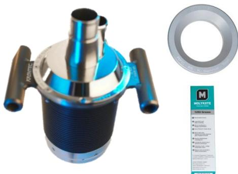
We recommend greasing the o-rings of the coupler with “Molykote 1292” after every race. Please use the following tool to open the nipple: **RFC-88-K-Service-Tool** (Figure 1).
